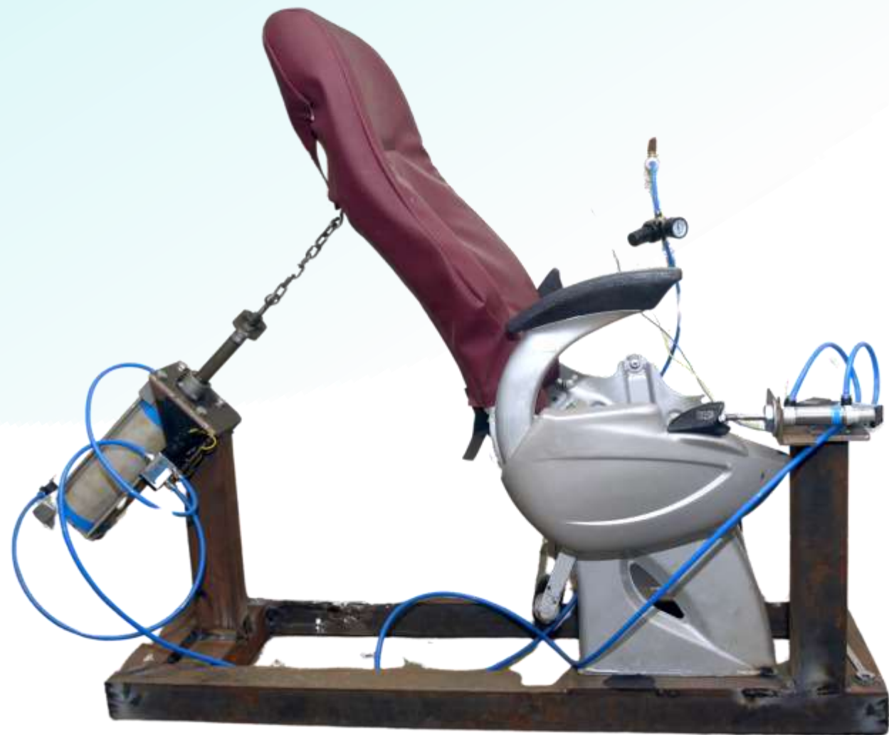
SEAT GAS SPRING TESTING RIG
